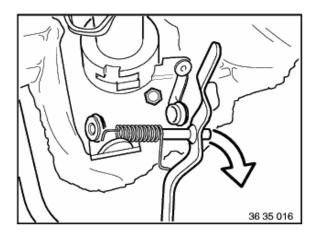
Disconnect return spring. Slide accelerator-lever shaft to the left and remove.
