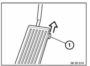
Press off locking washer (1). Disconnect pedal.
